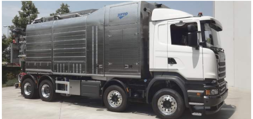
Equipment for extraction and conveyance of liquids and sewage from purging septic tanks
