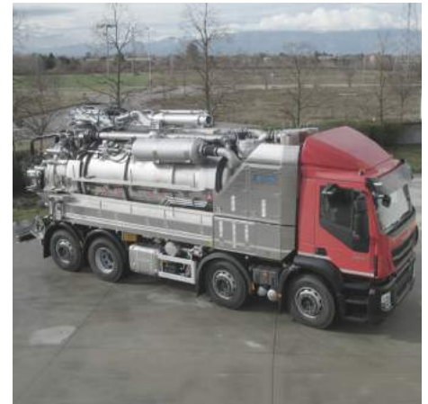
Example of a VJC outfitting with two PVT1000 (140000 l/min)
