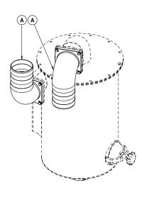
DL cyclone secondary shutoff (mild steel) - code 14450 026 E0
