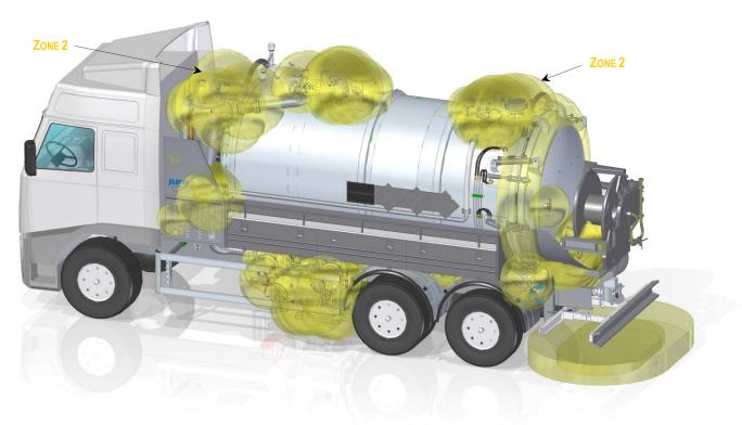
The extension, however limited, of areas with a potentially explosive atmosphere, is the result of a careful selection of materials that make up the ES, and of an innovative ventilation system of the tank and vacuum line, based on a
