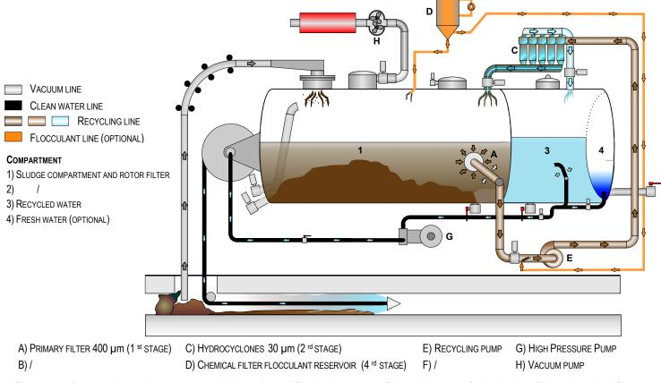
The compart. 4 corresponds to a clean water reservoir that can be used for cleaning purposes of the working area or for the cleaning of the equipment it self.
